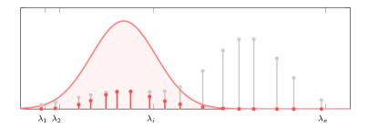
Filter banks scatter the energy of signal x into the signals  $z^{f}$  at the output of the filters.
