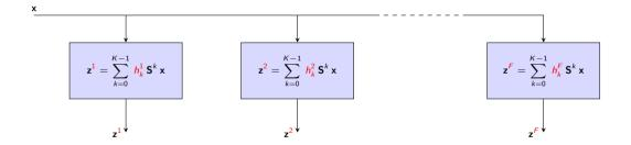
We would now like to process multiple feature graph signals. Process each feature with a filterbank.
